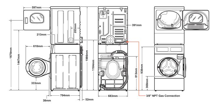
\*All Speed Queen dryers need to be vented to atmosphere (vented outside), please contact 1300 927 437 for venting solutions. \*\*Max ducting length 19.8mtr, reducing by 3mtrs for each 90deg bend.
